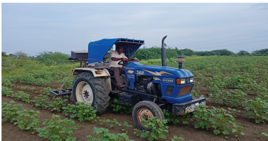
Plate 5 : Variable rate fertilizer application in cotton crop (30 DAS) at Fatehpur village, Raichur district
