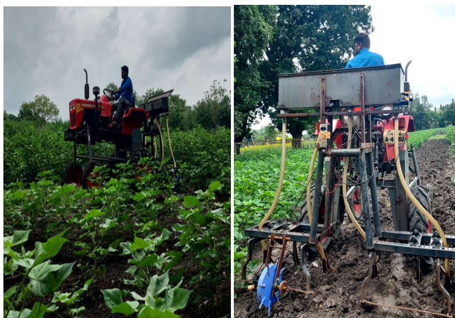
Plate 6 : Variable rate fertilizer application with high clearance tractor in cotton crop (60 DAS) at Fatehpur village, Raichur district
