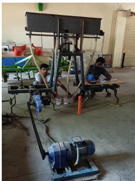
Plate 2 : Laboratory evaluation of variable rate fertilizer applicator at Farm Machinery Testing Centre UAS, Raichur
