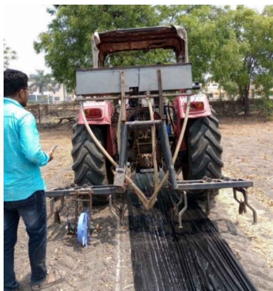
Plate 4 : Open field testing of variable rate fertilizer applicator at CAE, Research farm
